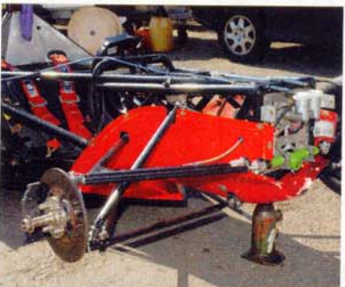
The Speads has inboard suspension and sports cross-drilled Alcon brakes
