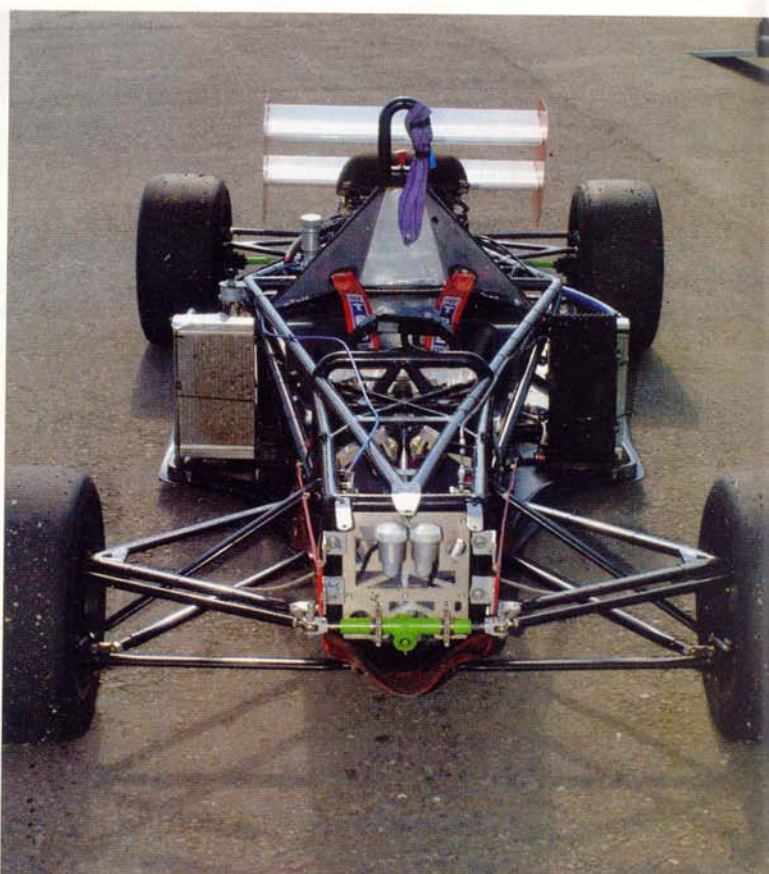
The diamond-shaped chassis frame is a highly complex piece of race engineering
